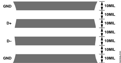
Figure 20. Arrangement of Signal Tracks
